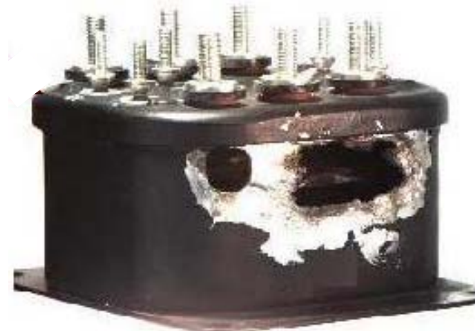
Damage from whiskers induced metal vapor arc in relay
